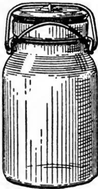
Fig. 7. Position of clamp during sterilization.
