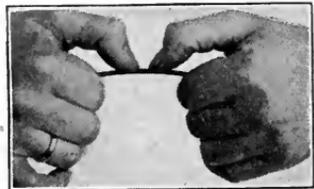
Bending the Ball to Tighten It
